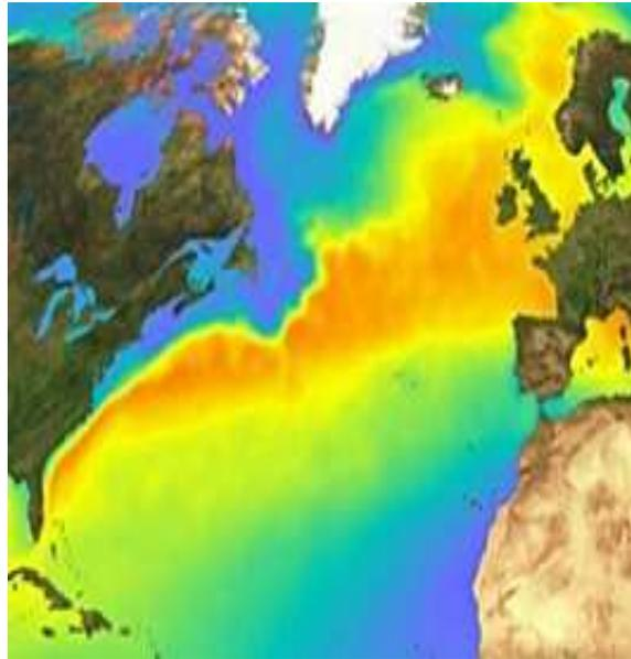
Orange color indicates the greatest amount of heat given off from the water to the atmosphere
